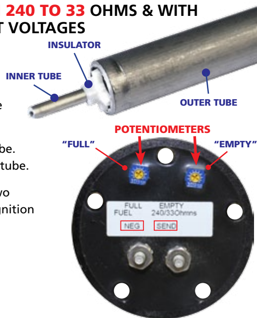
KS225 2-TERMINAL SENDER WITH POTENTIOMETERS (Power from Gauge)
