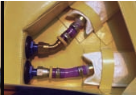
Sump with Dual Filtered Pick-Ups
