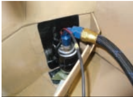
Open-Top Fuel Trap with Door and Pump
