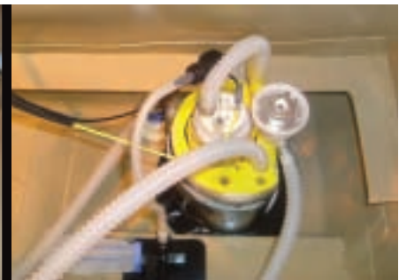
Adapted OEM Road Car Pump Module to ATL Bladder
