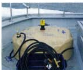
Fuel bladders let you extend your range, then fold up and stow away when you reach your destination.
