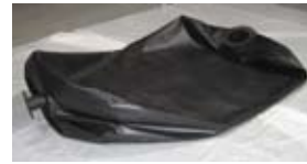
Bladder is Laid Out for Visual Inspection Prior to Installation
