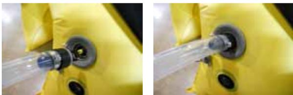
Insert ATL Inflation Device and Give 1/2 Turn Clockwise to Open Spring-Loaded Valve. Apply Low Pressure Air Source to End of Clear Hose to Inflate Support Tubes.
