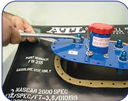
2 Remove fill plate with a wrench or socket. Lift plate slightly to access the existing pick-up hoses. Use two wrenches to disconnect pick-up hoses.
