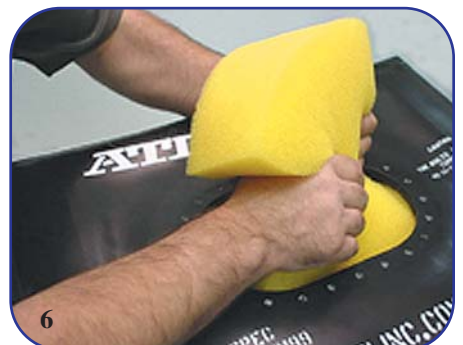
6 Carefully remove safety foam baffling. NOTE! before removal, flush cell with water to prevent a possible flash fire due to static electric charges. Let foam dry.
