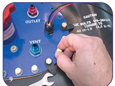
9 Once you are assured that there are no kinks or pinched wires, lower fill plate and begin bolting (with tabs). Tighten bolts to 40 Inch-lbs. Fuel Cell portion is done!
