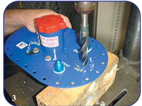
3 Drill an 11/16” (17mm) hole for the wire thru-fitting (Part# TF604). On TF195 plates, place fitting near vent to save open area for level sender option.
